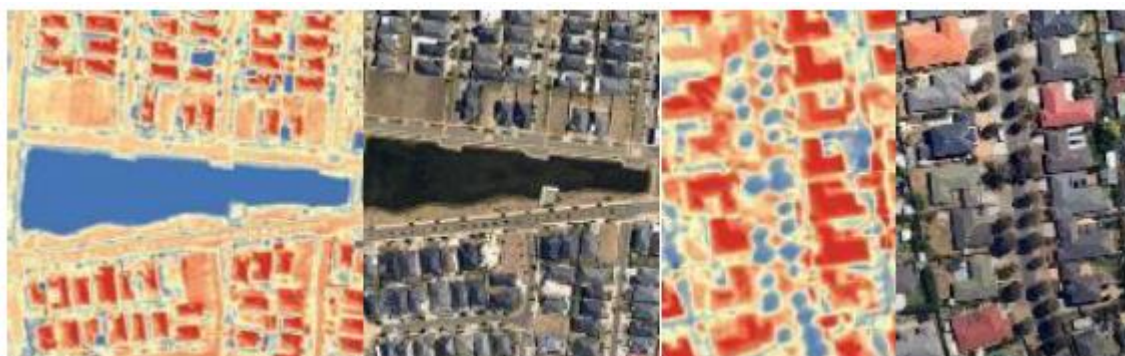
Thermal imagery of water body (left: 64 Scrubwren Dr, Williams Landing) and tree lined street (right: 17 Wattle Grove, Point Cook) Comparison of irrigated (~32°C) and unirrigated ground cover (~45°C) (19 Kingsley Ave, Point Cook) Source: Wyndham Integrated Water Cycle Management Plan (page 32)
