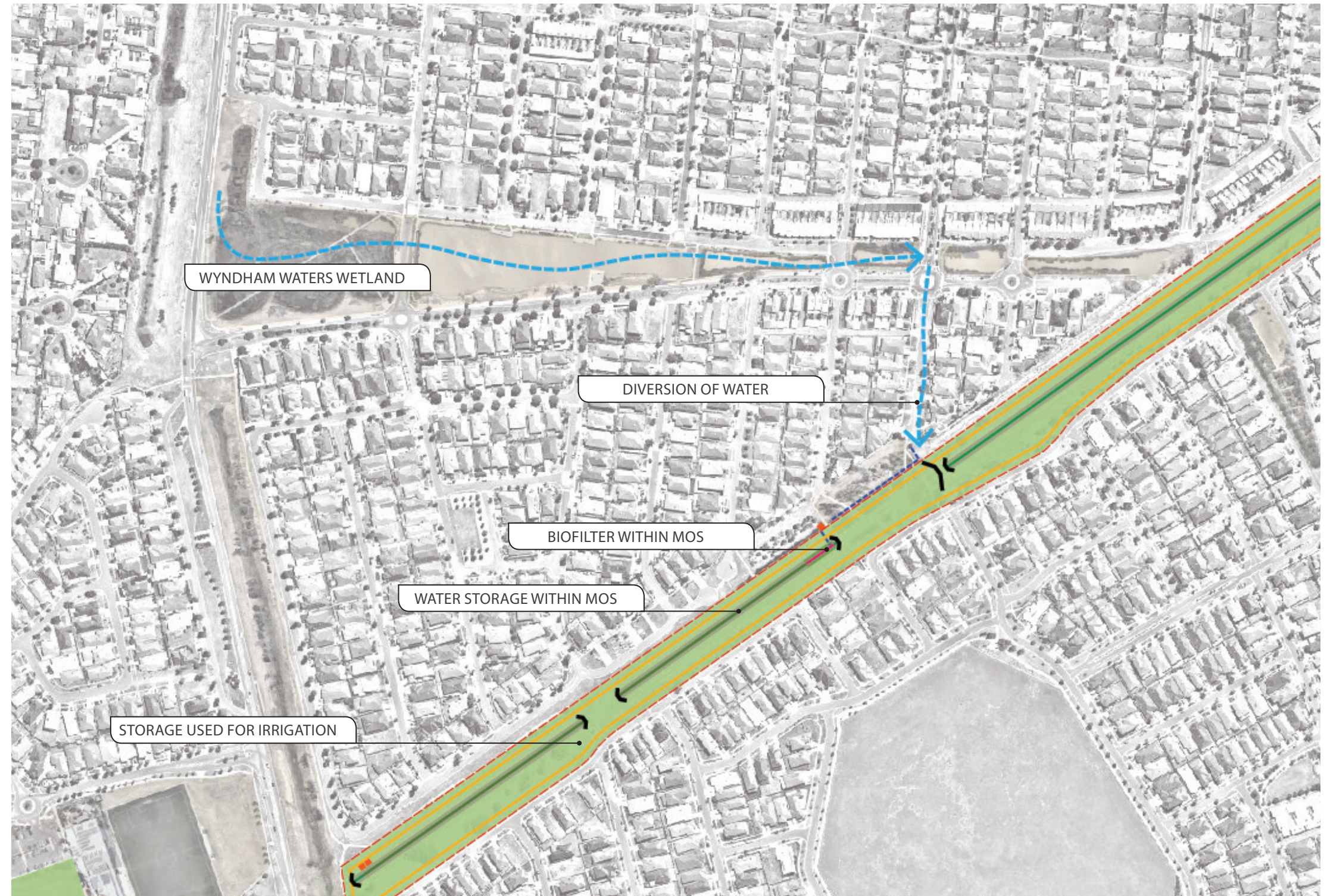
DIAGRAM SHOWING WATER HARVESTING FROM WYNDHAM WATERS
